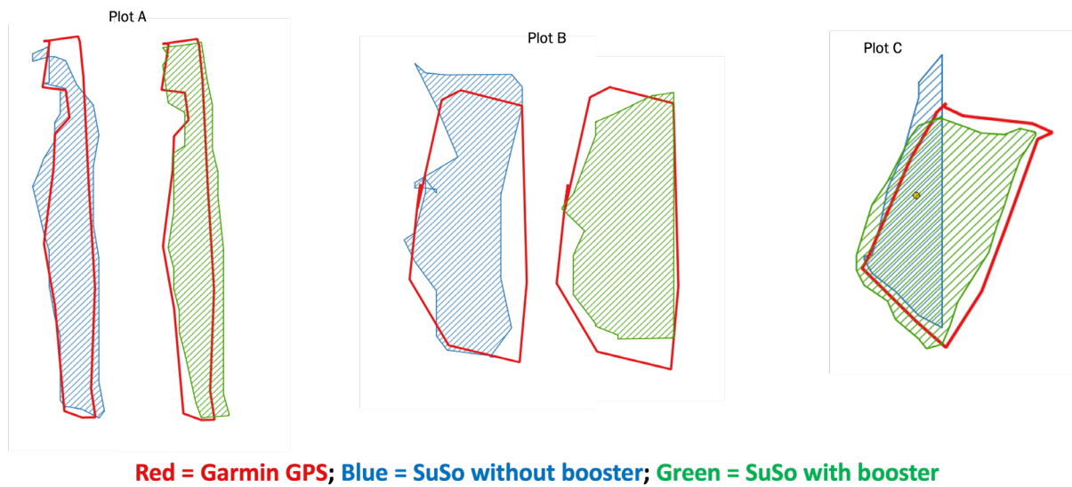
Figure 1. Comparison of plot boundaries measured using Garmin GPS, SuSo without booster, and SuSo with booster.
